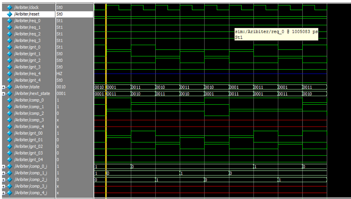
Fig10: simulation waveform for arbiter when all are request high
